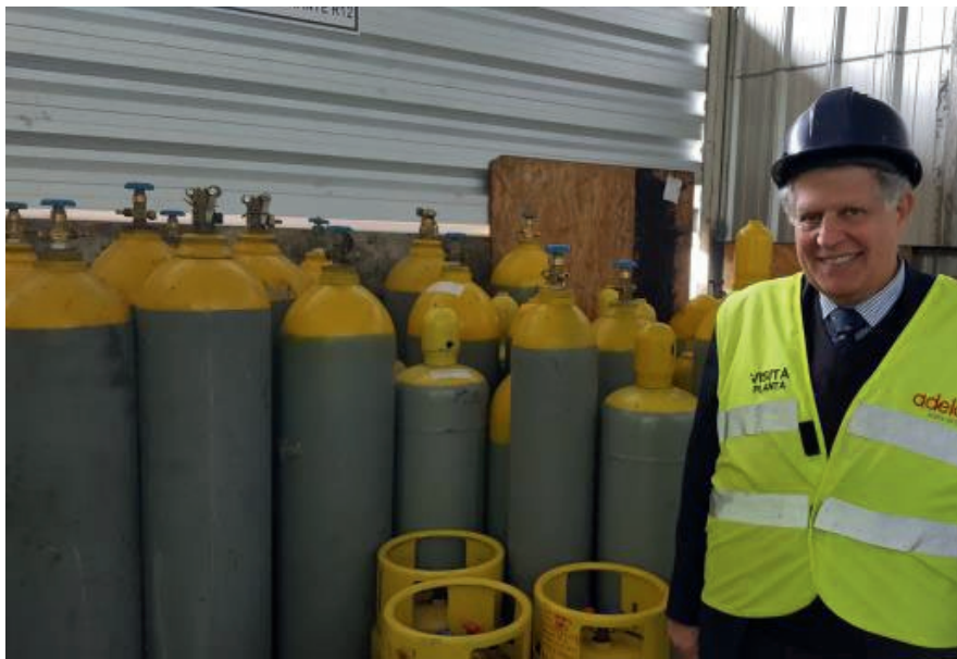
ECUADOR: R134 recovered and stored for destruction at Cement plant
